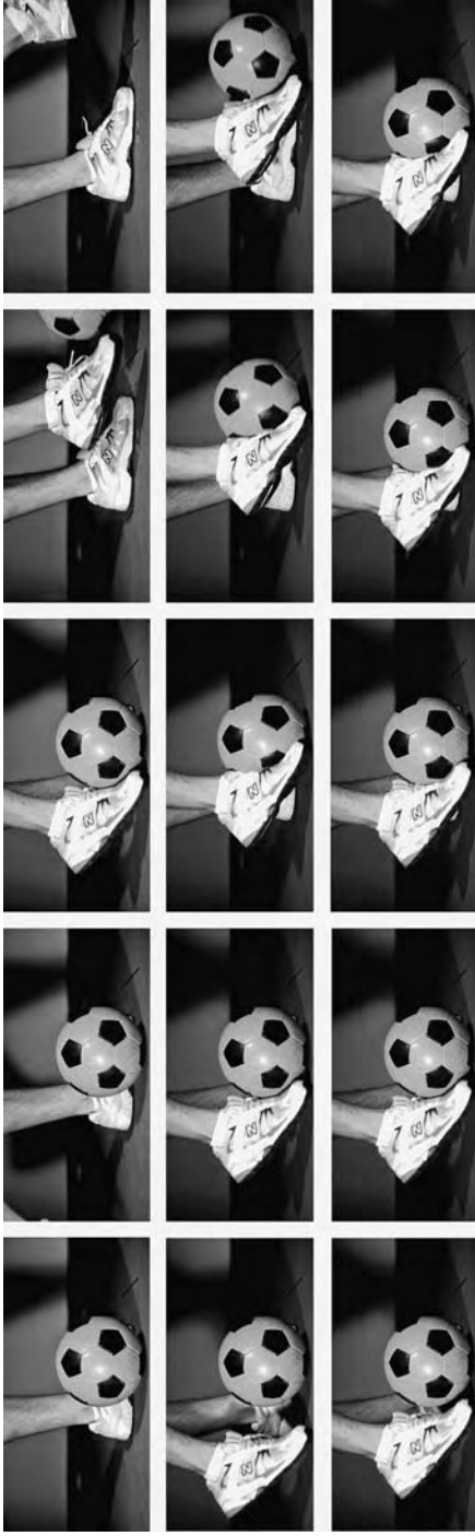
Figure 2.4 The effect of camera frame rate on the recording of a football kick. At 50 Hz (top row) the foot is only seen in contact with the ball for one image; at 250 Hz (middle row) the foot remains in contact for four images; at 1000 Hz (bottom row) the foot is in contact for sixteen images (not all images shown)
